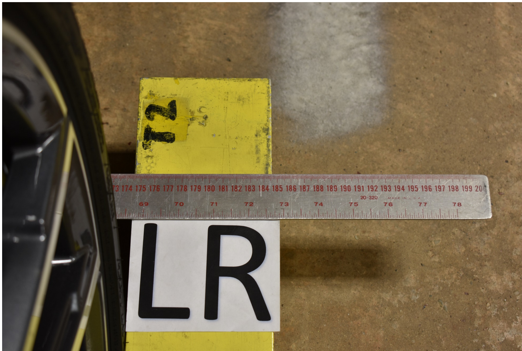
FIGURE 5.23 REAR LEFT TIRE REAR MEASUREMENT
